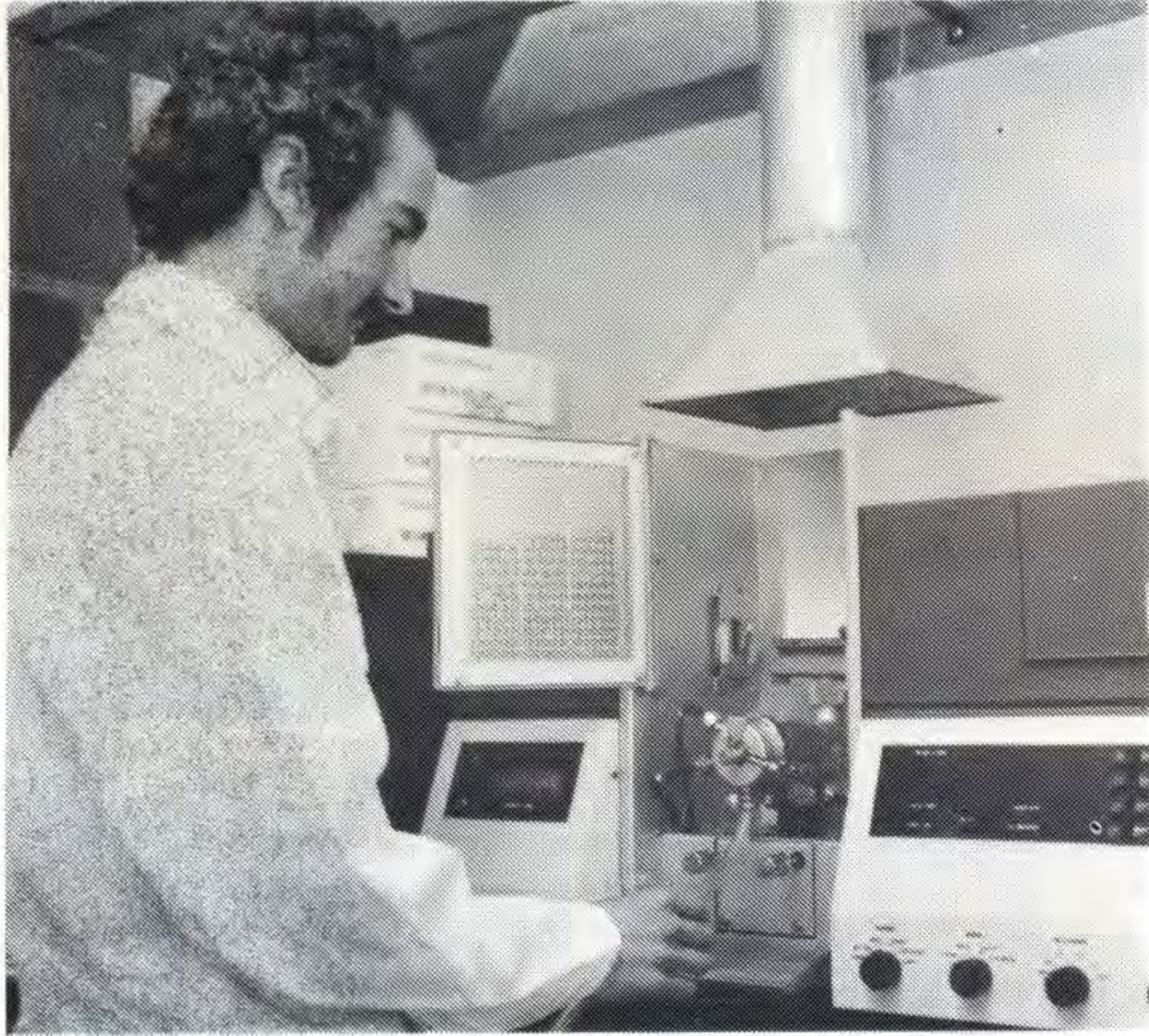
Max Griffin, Officer-in-charge of the Water Test Group is pictured (right) operating the atomic absorption spectrometer in the Morwell Briquetting and Power Installation's chemistry laboratory.
