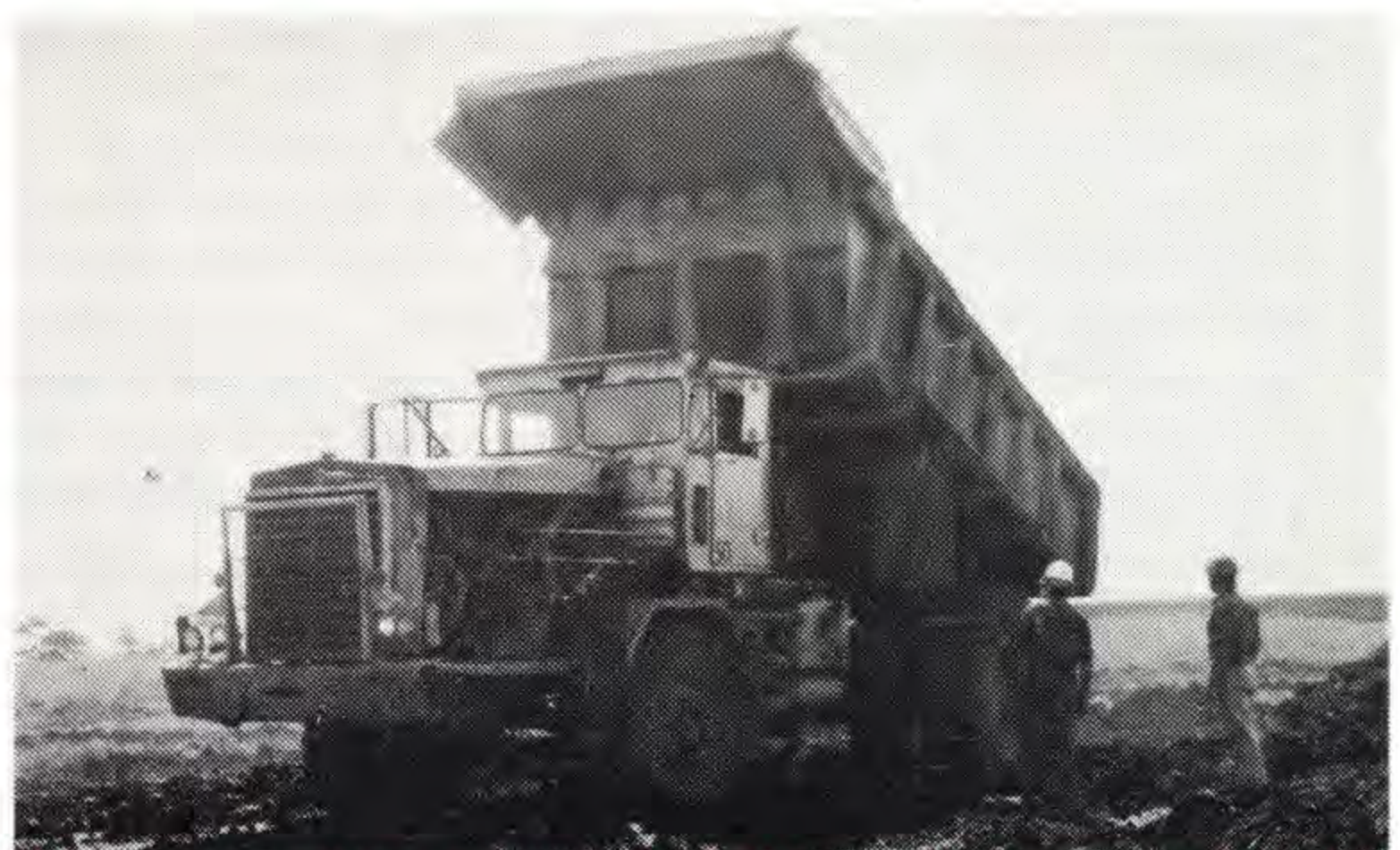
The two workers (above) look like midgets compared with the huge 45 tonne Euclid truck which is 18 feet high. There were 13 Euclid trucks working on the Morwell River project at one stage.
