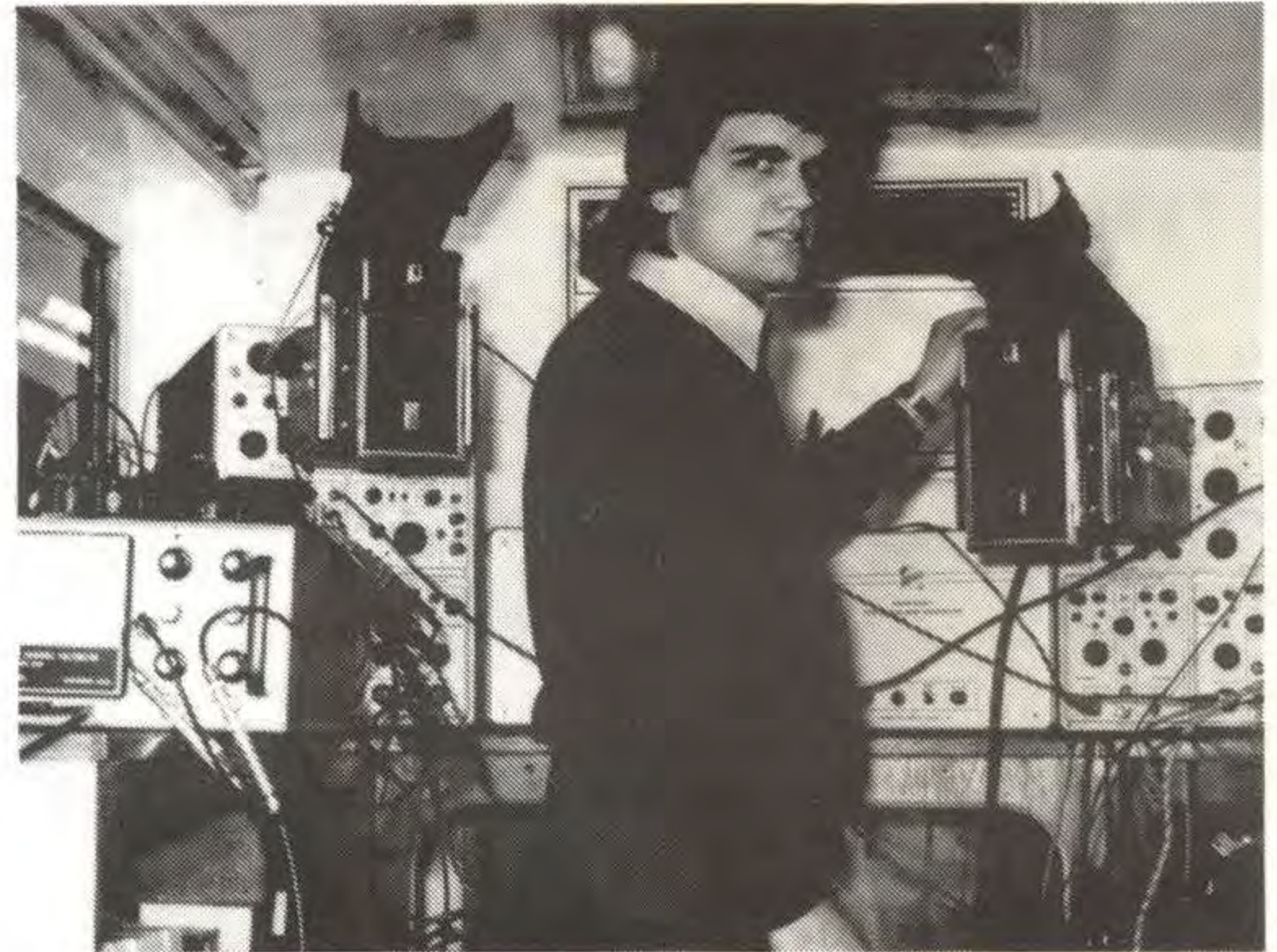
Engineer, Alan Smith (above) is pictured observing the high speed oscilloscopes used in recording the switching surge voltages. The memory voltmeter is in the left hand side of the picture.
